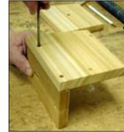
**2** Step 2: attaching side to back - Stand the back on edge with "keyhole" for mounting facing out. The side pieces have pre-drilled holes; set one side on the edge of the back so that the top of the side will be flush with the beveled edge of back. Insert two screws and tighten. Fun, huh?
