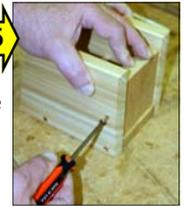
**6** Step 6: front panel - install front panel with entrance hole closest to floor - this allows warmer air inside roosting box to stay inside keeping chickadee warm in cold winter months.
