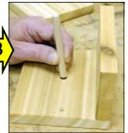
**3** Step 3: installing perch - insert 3/8" diameter perch in pocket hole on side.
