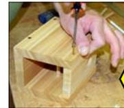
**5** Step 5: floor - Insert floor between sides roughly 1/4" above the bottom of sides and back. Press floor into back while attaching screws thru sides, then flip & screw thru back.
