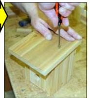
**8** Step 8: closure latch - place roosting box on its back to install "L-shaped shoulder hook" which will serve as a latch to keep front panel closed.
