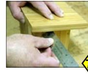
**7** Step 7: roof - place roosting box upright to install roof. Position roof flush along back and equidistance (see 7b) on both sides; attach screws. The roosting box can be attached to a tree, deck or fence railing using mounting keyhole. Or, the box can be pole mounted... see [www.jjcardinal.com/accessories.htm](http://www.jjcardinal.com/accessories.htm) for details about mounting flanges and poles.
